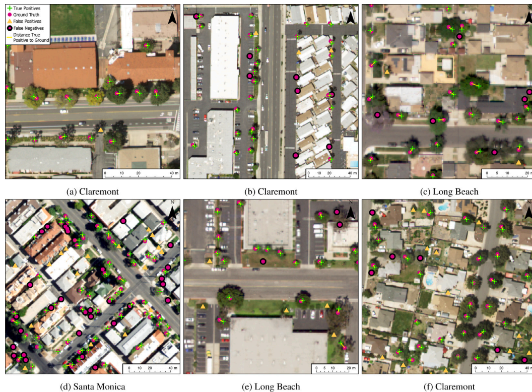
Fig. 4. Example results from our tree detection method on images from Southern California 2020 test set. The method is able to detect and accurately localize most of the trees in the images. Some areas contain examples of missed detections of trees with small canopies and shrubs being confused with trees.
